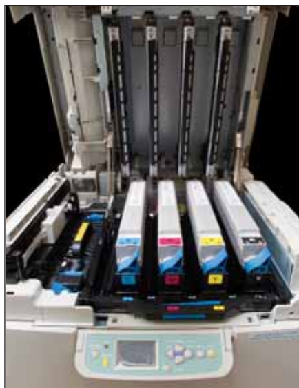
With the cover up you can see the flat paper path under the toner cartridges.
